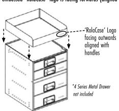
B Secure the Top Tray to the metal cabinet using the 4x dog head phillips screws supplied, this can be done manually with a Philips screwdriver however it is much easier using a cordless drill with a P3 bit on a low torque setting to ensure you do not strip the thread
