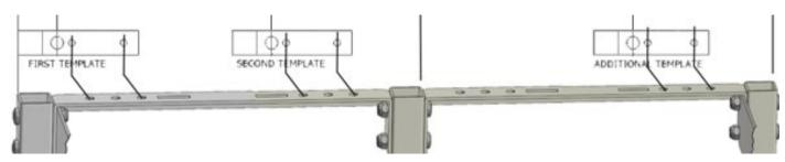
Q Now that you have marked three holes per tongue on the upper frame body of the vehicle, move the assembled frame bays out of the way for convenience and carefully drill the 13mm-9/16" hole and 7mm-5/16" holes as per the following template:
