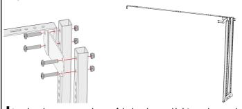
Introduce the extension to the top of the loosely assembled Starter bay completed in the previous step. Note that this Extender HD Upper Angle Bar must be secured to the correct side of the Starter Bay so that the final intended configuration can be achieved. Remove the two finger tight nuts on the end of the frame and slide the Upper Angle bar over the screws and then return the nuts to create the extension Refer to images below:
