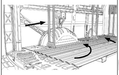
Now that the assembled bays are in the cargo area of the vehicle, carefully move the unit into the desired position and check that this position does not or will interfere with any other vehicle systems or the standard operations of the vehicle. The next steps will explain the assembly of the Universal Anchors and how to attach them from the body of the vehicle to the HD Upper Angle Bar.
