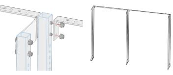
At this point you should have two shelving bays secured together outside of the vehicle. Double check that all parts are in the correct location and cross reference against the assembly images provided. Once you are satisfied that every part is in the correct location, proceed to tighten all the nuts and bolts that were left finger tight in the previous steps. The end result should produce two frame bays fully assembled together as shown above
