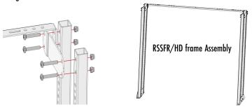
■ Locate the second HD Upper Angle Bar and third set of posts supplied in the Extender Kit and assemble the HD Brackets and the Upper Angle Bar #2 using steps 1 to 3 making sure the Upper Angle Bar is in the direction you wish to extend. Refer to images below:
